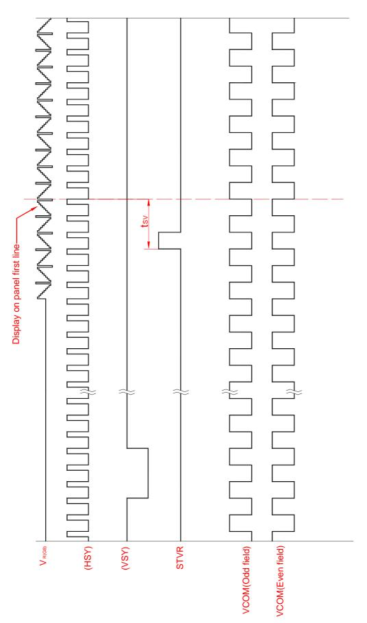
Fig.6-(b) Vertical timing (From down to up)
